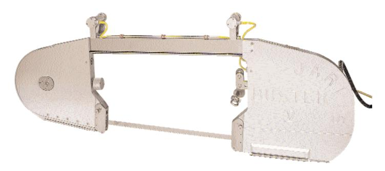
The Jarvis Model Buster V Loin Drop - electrically powered bandsaw for beef loin dropping (quartering).
